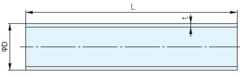
Diagram showing dimensions for JIS K 6776 pipes. Key dimensions include: φD (Nominal Diameter), L (Length), and thickness t.
